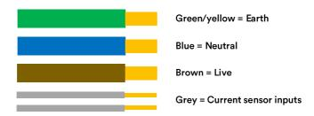
The input lead is one metre long and the supply conductors are 6mm<sup>2</sup> copper. They need to be terminated to a junction box, isolator or direct into a consumer unit.
