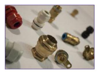
CW Glands are for use with all types of Single Wire Armour (SWA) cable providing mechanical cable retention and electrical continuity via armour wire termination. Also provides a seal for the outer sheath of the cable which gives it the IP protection. These are used both indoor and outdoor.
