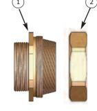
4. While continuing to push the cable forward to maintain contact between the armour and the cone, tighten the Nut (2) by hand to engage the armour. Hold the Entry Component (1) with a spanner and tighten the Nut (2) using a spanner until the armour is secured.
